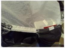
Push the batten back somewhat and release the end from the pocket, then remove it entirely. Transfer the total length precisely to the replacement material (supplied) and cut a new length. File the ends of the new batten and cover them with tape. Push the new batten into place and secure.
