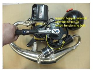
fit Inbus socket into the center bolt of the drive wheel front as shown. Now start to turn slowly in anticlockwise direction (!, never in the other way) until you reach the set torque
