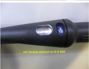
set your torque wrench to 8-9 NM, use a Inbus type hexagon socket 8mm (metric)
