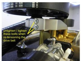
Untighten the shown bolts, open one after the other in small steps, until you can easily turn the drive wheel eccentric shaft
