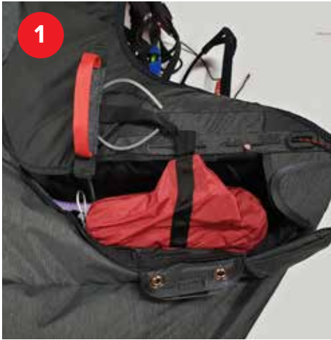
1 After connecting the rescue to rescue bridle, insert rescue with handle facing UP
