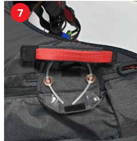
7 Remove the paracord slowly, place the handle flap on the velcro as shown
