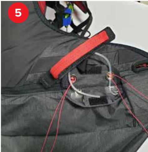
5 Pass the handle wires through the closure loops
