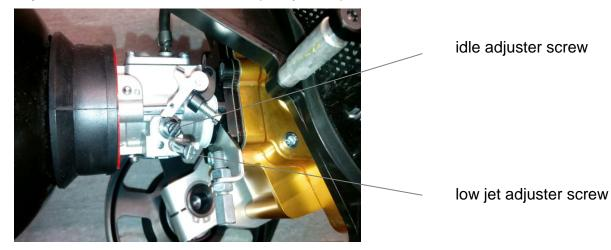
Idle adjuster screw - for proper setting proceed as follows;
