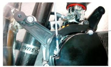
remove cable binding after starter rope installation
