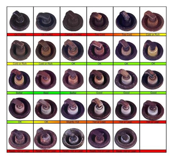
The EOS engine's standard setting is adjusted to rather a bit to rich run in order to have a safe engine run. The main adjustment is made by the selection of a proper main jet inserted into the carburetor. The low jet adjuster screw helping for a proper setting in low and medium RPM's but not changing the combustion temperature and condition under high and full RPM.
