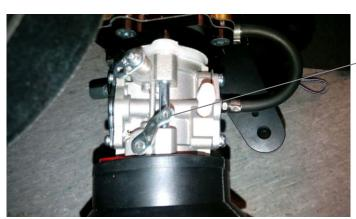
choke lever open position closed/activated
