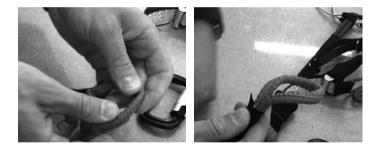
Then fasten each spreader with an anchor hitch to a closed FORAS carabiner.
