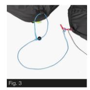
For the first step in fitting a Light speedbag release the grey adjustment section at the upper ends from the two lower blue speedbag lines. To do this loosen the kits knots of the blue speedbag lines and pull these off the grey adjustment lines. Now fasten the two grey adjustment lines with kite knots direct to the black loops on the edge of the seat surface. Then fasten both lower blue speedbag lines to the grey adjustment lines, again with kite knots.
