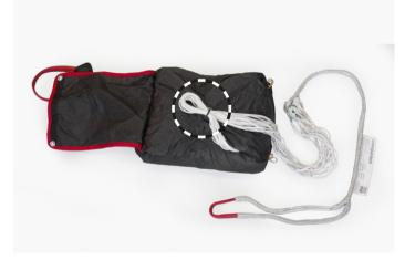
Now close the outer container flap (red border) with two similar line loops (5 to 6 cm). These two line loops are secured in the two attached rubber bands though their eyelets on the outer flap.
