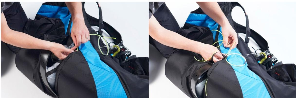
Close the large black plastic flap using the cord and block the elastic loop using the longest pin, having it pass first through the hole just under the handle insertion, then in the elastic loop and finally in the hole located after the elastic strap. Then remove the thin cord.
