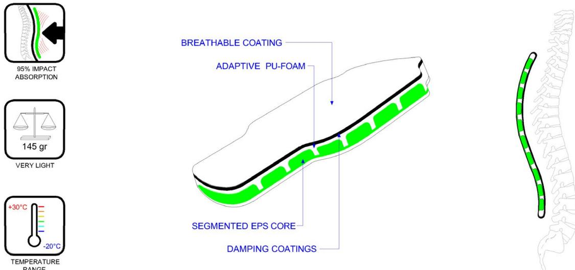
The absorption effect of the back protector reaches approximately the required value with a residual force of only 975 kN. This means that approximately 94% of the impact energy is absorbed. The materials and their protective function are TÜV SÜD approved in accordance with European standard EU-Norm 89 /686 / EWG and have been tested/certified as personal protection equipment category 2 (PSA). They also meet standard TÜV/GS on product safety.
