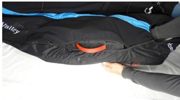
Insert the metal handle pins into the elastic loops. The cord must be removed at the end of this stage and must be extracted slowly in order to avoid damaging the elastic loops due to excessive friction between the parts. At the end, the handle should be inserted into its housing. Ensure the handle cover lies flat and under the Lycra flap, hooking it to the Velcro.
