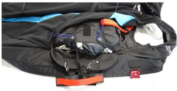
Introduce a thin rope (1 or 2 mm diameter) into each elastic loop which you will use to help close the container. Introduce the elastic loops into the two smaller eyelets. Follow the closing order of the various flaps visible in the photos.
