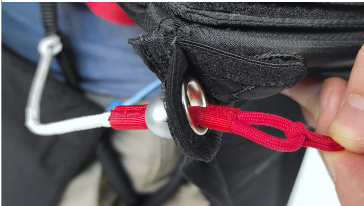
3. Push the T-piece through the latch.
