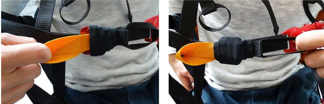
At shoulder strap height, there is a small hook that acts as a shoulder strap fastener and prevents the shoulder straps from sliding off the shoulders during take-off. The plastic coupling also holds a practical whistle which can be helpful in the event of an emergency.
