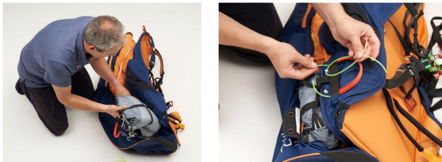
Take the bridle cover zip and the second zip that closes the other end of the container to their start point under the emergency parachute handle. Close the zip on both sides about 20 cm. Close the external part of the container as shown in the photo, taking care during this phase that none of the zips open. Insert the two plastic yellow pins into the elastic loops and then under the cover arranged between the two.
