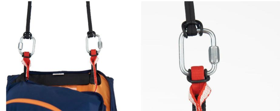
The two connections should be made using screw-lock karabiners with a breaking strength of at least 1,400 kg. It is important to verify that the length of the bridle is sufficient to position the reserve parachute inside the harness pocket, and that there is sufficient play to enable the parachute to be taken out of the pocket without causing the reserve parachute deployment bag itself to open during extraction.
