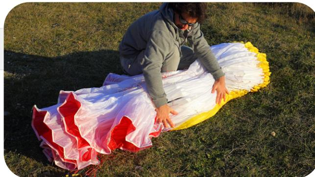
**Step 4.** Once the LE and TE of the wing have been sorted, turn the whole wing on its side.
