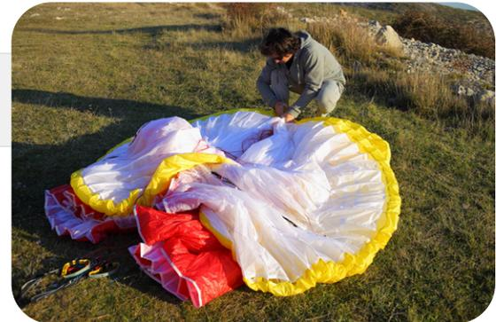
**Step 2.** Group leading edge (LE) plastic reinforcements with the A tabs roughly aligned. Make sure the plastic reinforcements lay side by side. Note the glider is NOT folded in half; it is folded as a complete concertina from wing tip to wing tip.
