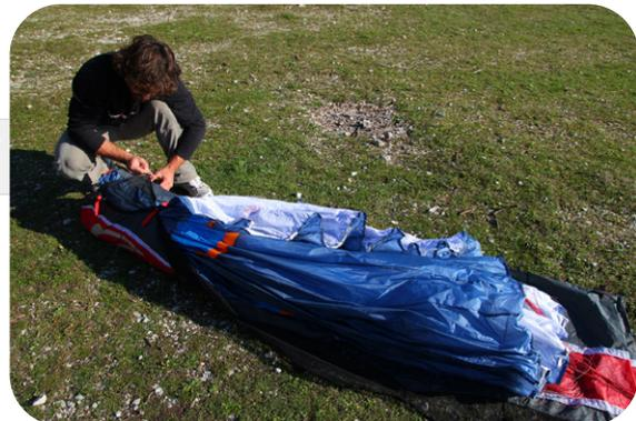
**Step 8.** Lay the Folding Pillow in place and make the fold of the LE around it. Use 2 folds.
