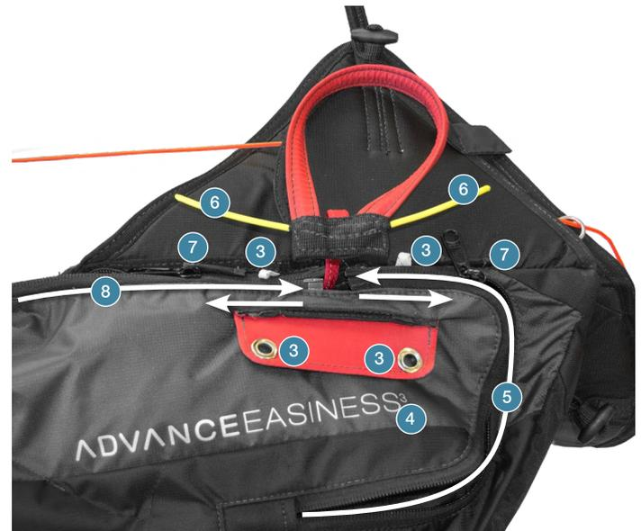
Tuck the base of the reserve handle into its neoprene pocket. 9 Then close the right hand zipper 5 by running it all the way round, into its zipper garage. Close the left hand zip 8: run it up the side of the harness to the top of the harness – this closes the V-connection channel – and be sure to park it in its garage
