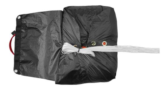
Close the last flap of the container with two line loops of equal length (5 to 6 cm). These final loops are held by two elastics that pass through the eyelets of the outer flap of the container. The two elastics are pre-assembled at the factory.
