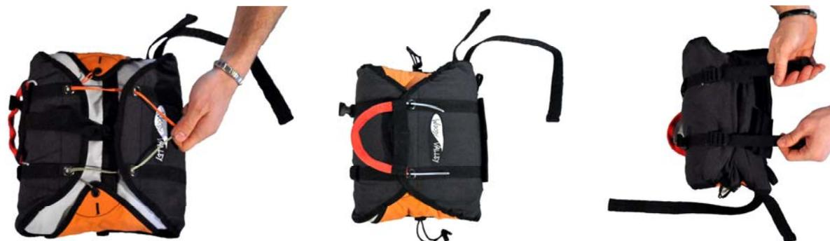
Push the plastic pins on the handle into the elastic loops and under the transparent cover. It is essential to remove the cord after this operation. The cord should be pulled out slowly in order not to damage the elastic loops by excessive friction. Lastly, the handle should be positioned under the two cover loops. The reserve parachute and harness are joined by means of Velcro strips, and a loop which is hooked onto the main karabiner.
