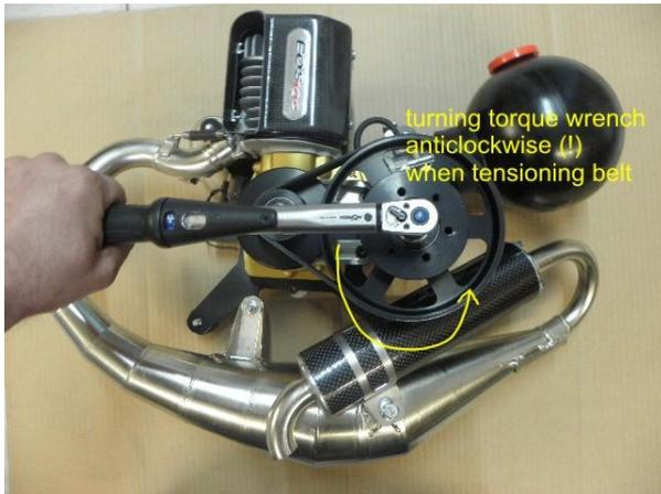
fit Inbus socket into the center bolt of the drive wheel front as shown. Now start to turn slowly in anticlockwise direction (!, never in the other way) until you reach the set torque
