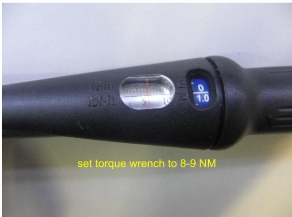
set your torque wrench to 8-9 NM, use a Inbus type hexagon socket 8mm (metric)
