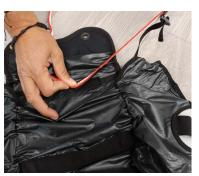
The container "V"bridle has a Velcro fastener so that it can be attached to the container once the "V"bridle is connected. Place the parachute and its bundle in the container, keeping the handle facing upwards. To close the container flaps, slide a thin cord (such as a paragliding cord) into each elastic loop, which will help you close the container.
