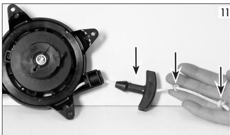
**⚠ ATTENTION:** verify that the return spring does not reach the end of the stroke. Pull the rope completely and turn the wheel again to check that it can make at least one turn before stopping. This test is very important because the spring hasn't been studied to reach the end of the stroke and, if it happens, the spring will break. Reassemble the starter in the engine and tight the 4 screws (M5) with strength (see the tightening torque values table).
