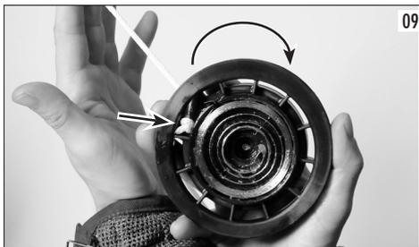
Now insert the plastic wheel in its housing again, and check through the hole that the internal spring hook is perfectly coupled (Photo 10), place the springs, the teeth for the starter jaw and screw the cover again using medium thread-locker.
