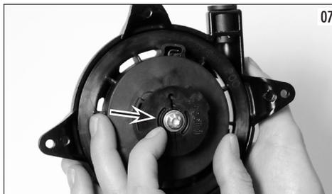
**⚠ ATTENTION!** Under the cover there are two teeth for the starter jaw (check their condition and if worn replace them), under them 2 small calipers. Be very careful not to lose these small parts. Prepare the new rope and tie a knot at the top. Remove the plastic wheel and the old rope. Put the new rope in its hole (photo 8), wind up the rope on the wheel (according to the entrance sense of the rope on the wheel (Photo 9).
