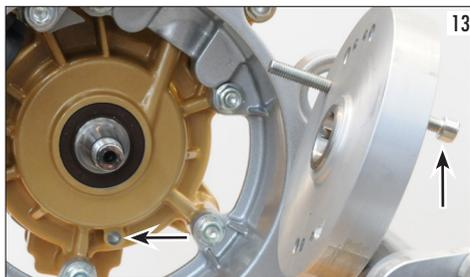
Screw the flywheel nut without locking it so that the crankshaft can rotate in the flywheel. Screw the dial gauge support into the spark plug hose, insert the dial gauge and move the piston to the top dead centre. Now reset the dial gauge and rotate the crankshaft anti-clockwise of 1,7 mm towards the flywheel sense (see arrow in photo 14).
