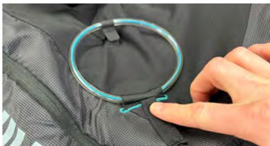
When all is set, train yourself to know where the deployment handle is and always check your parachute is secured before going to fly.
