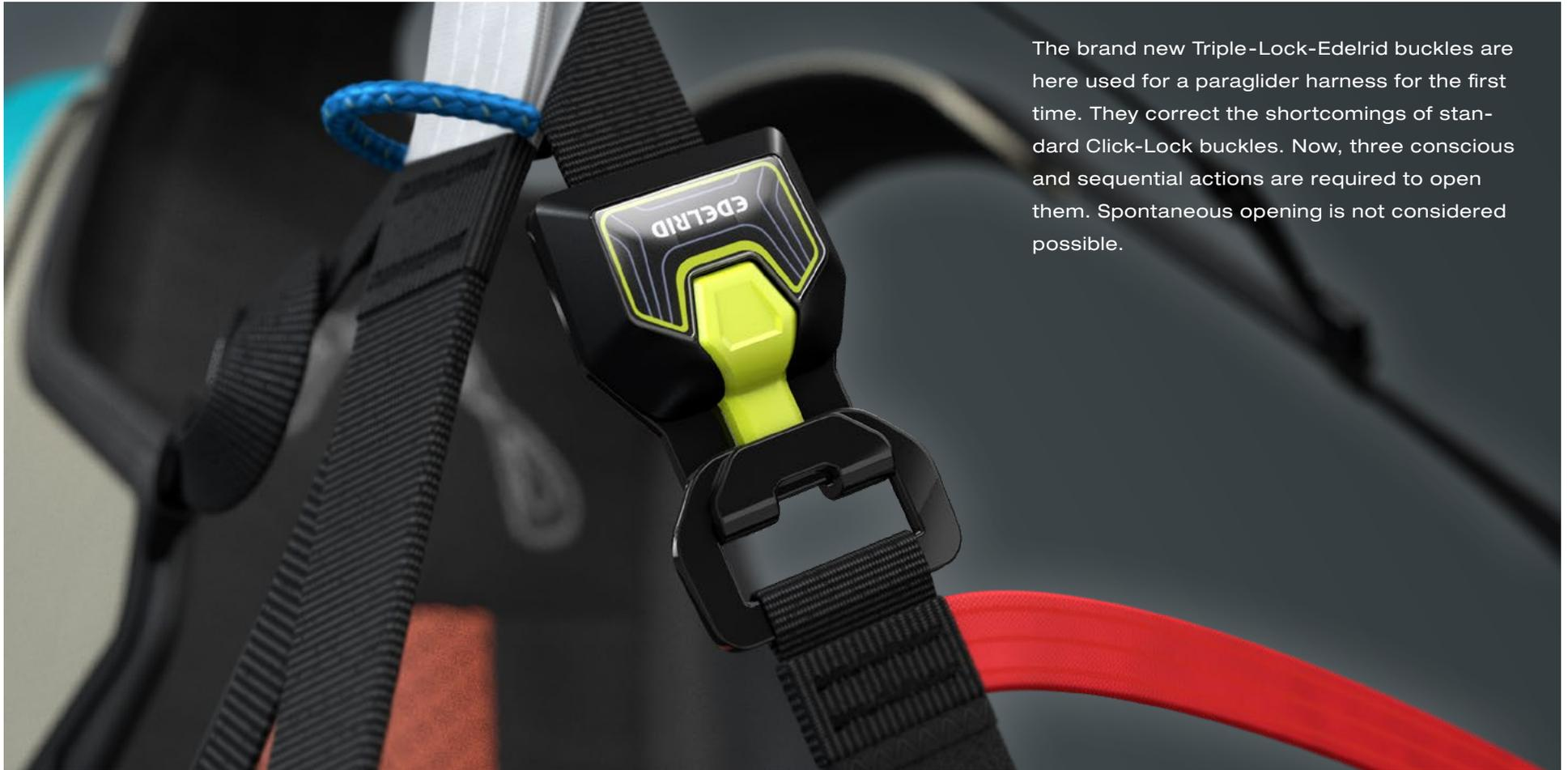
The brand new Triple-Lock-Edelrid buckles are here used for a paraglider harness for the first time. They correct the shortcomings of standard Click-Lock buckles. Now, three conscious and sequential actions are required to open them. Spontaneous opening is not considered possible.
