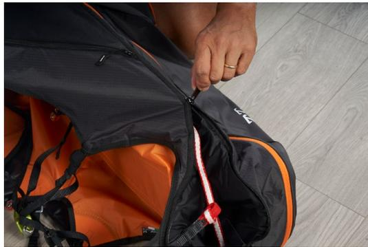
Take the bridle cover zip slider and the second zip slider that closes the other end of the container to their start point under the reserve parachute handle.
