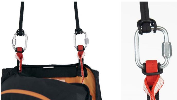
The two connections should be made using screw-lock snap-hooks with a breaking strength of at least 1,400 kg. It is important to make sure that the bridle is long enough to position the reserve parachute inside the harness pocket and that there is sufficient room to take the parachute out of the pocket without causing the reserve parachute deployment bag itself to open during extraction.
