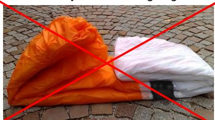
Do NOT fold the leading edge under, as shown here above.
