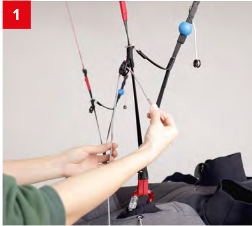
1 Once the riser speed line has been removed, pass the speedbar line through the top pulley
