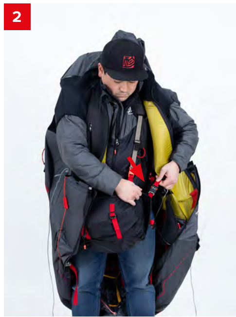
2 Connect the front support pillar metal buckle and adjust the volume of the container with the red straps
