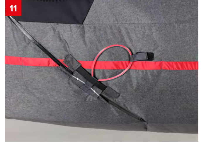
11 Stick the velcro to the outershell velcro to maintain the handle position in flight
