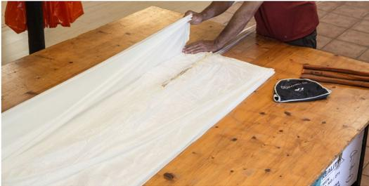
The left third is folded onto the middle and then the right third is folded under the middle. Do the same on top of the canopy.
