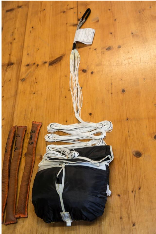
The suspension lines are sorted in three bundles, which are fixed by rubbers. These bundles are stored in the pocket of the container.
