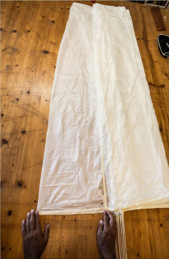
Put all the panels to the right side and fold over each panel from the right side onto left side like turning the pages in a book and pull the top of the opening outward..
