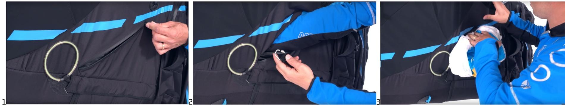
(1) "Anti-G" side pocket; (2) karabiner for attaching the drag chute bridle; (3-4) "Anti-G" stowage; (5) Example of extracting the drag chute; (6) "Anti-G" stowage.
