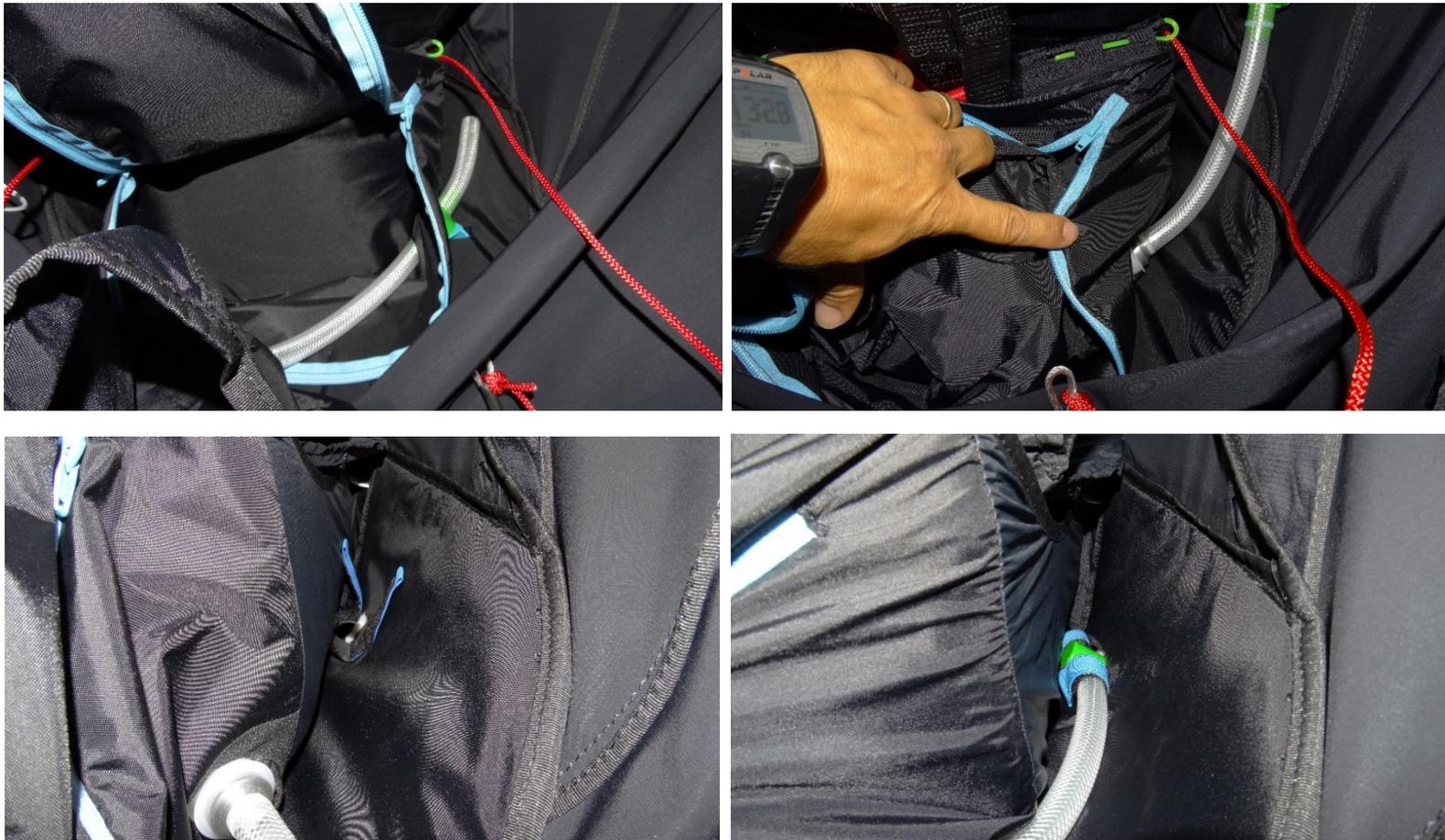
The ballast compartment is located beneath the seat. Open the zipper to access and insert the discharge tube into the hole on the right and install the ballast. Slide the tube into the sleeve on the side until it comes out of the other side. Lodge the tap in the hole and use the blue Velcro strap to secure the tube so that it remains in place.
