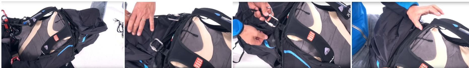
The two connections should be made using screw-lock karabiners with a breaking strength of at least 1,400 kg. It is important to verify that the length of the bridle is sufficient to position the reserve parachute inside the harness pocket, and that there is sufficient play to enable the parachute to be taken out of the pocket without causing the reserve parachute deployment bag to open during extraction.
