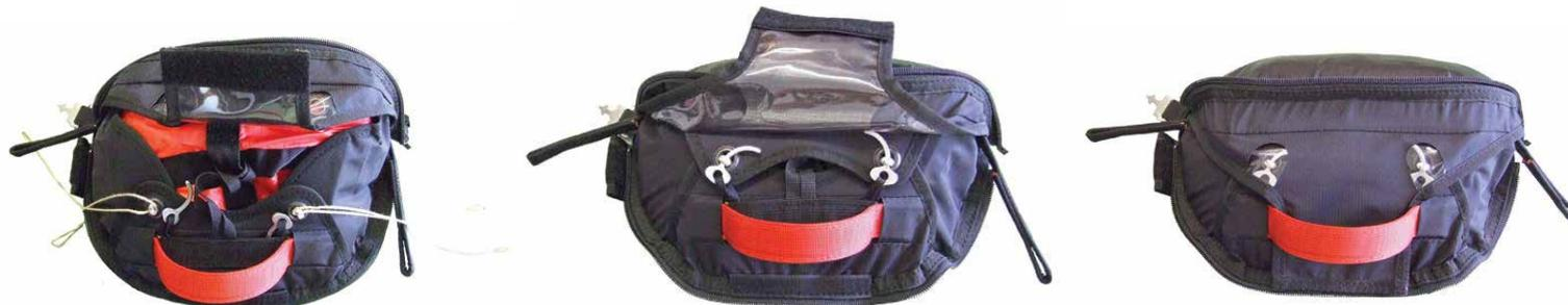
The container is connected using the special buckles and must be fastened to the leg-cover using the zipper. The parachute container houses the instrument compartment, which is also connected using a zipper.
