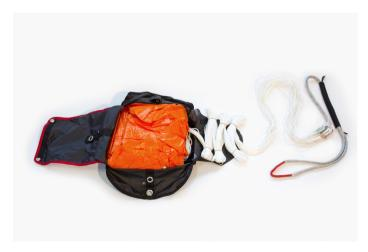
Close the container flap in the order indicated (1-3). Secure the final container flap (3) with a 5 to 6 cm line loop (ca. 3 finger widths). Now check the tension of the bungee loop and adjust if necessary. --> lift the package by the lines - the weight of the reserve should release the line loop.
